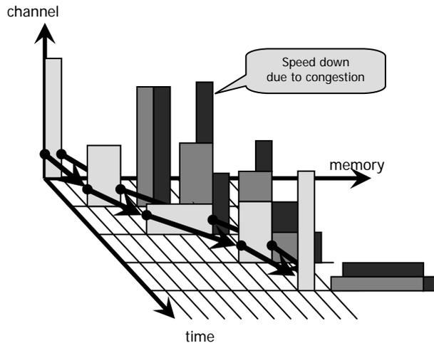
Fig. 2. Summed-up communication channels: A data transfer activity is initiated as a packet with narrow but high effect extent. Its effect extent gradually becomes wider but lower, and then returns to a narrow and low profile before reaching the destination. Loads of different packets are summed up.
