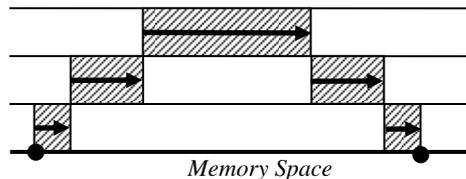
Fig. 1. Layered communication channels: A data transfer activity is initiated at the lowest level, goes to higher levels, and finally goes down again before reaching the destination.
